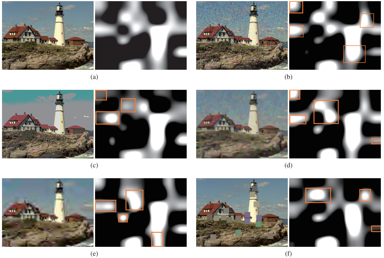
Fig. 1: The reference image from TID2008 database, and its five derived images, deteriorated by (b) spatially correlated noise, (c) quantization noise, (d) image denoising, (e) JPEG2000 compression, (f) local block-wise distortion respectively, along with their corresponding reconstructed images.
